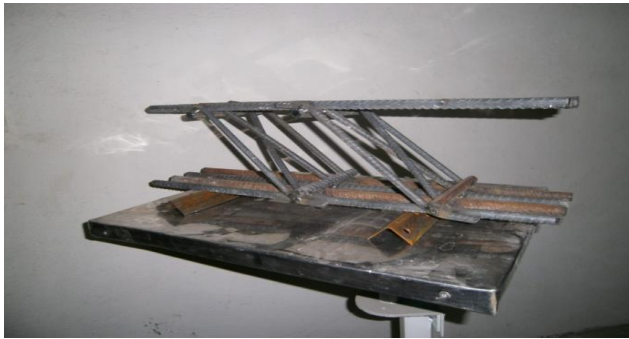
Rectangular swimmer bar system with cross bracings.
